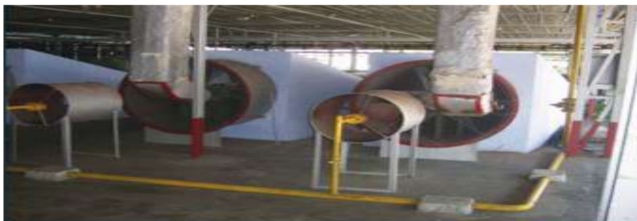
Figure 1: Withering Fan fitted along withering trough
