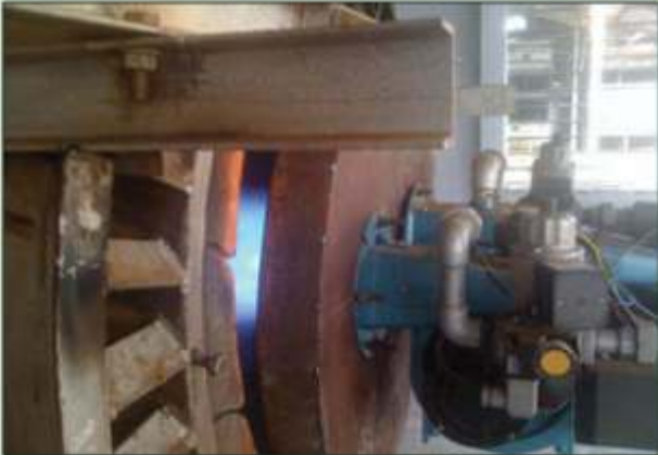
(Fig. 4b: View of the Gas Burners (2 Nos. to match the heat energy input) fitted on the DF heater)
