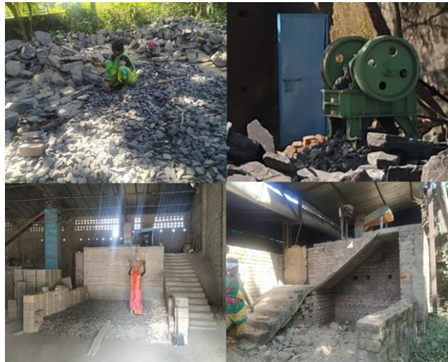
Figure 4.2.1a: Jaw crusher and disintegrator
