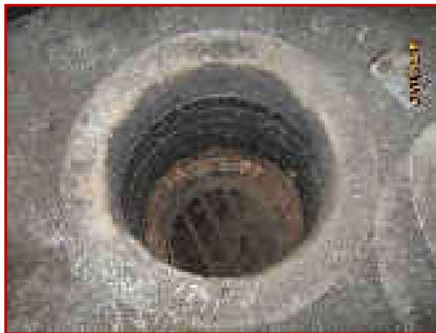
Figure 3.10: Insulation in conventional coal fired pit furnace
