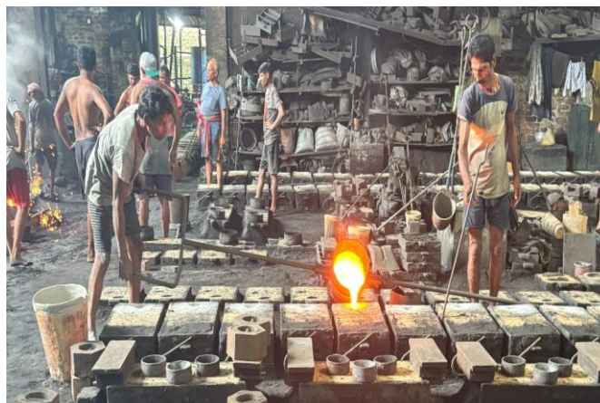
Figure 8: Pouring practices in Howrah foundry cluster
