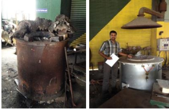
L-FO-fired furnace; R-Electrical conduction furnace
