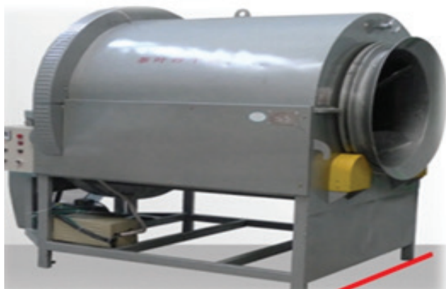
Figure 3. Withering fan with electric heating assembly
