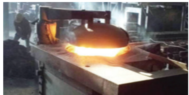
Deep dive in Rajkot foundry cluster: lid mechanism installed for induction furnace
