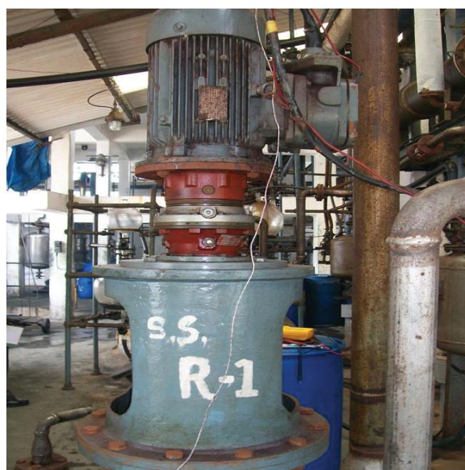
Vertical agitator driven reaction vessel
