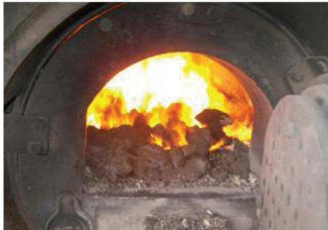
**Proper sizing of fuel to improve combustion efficiency**
