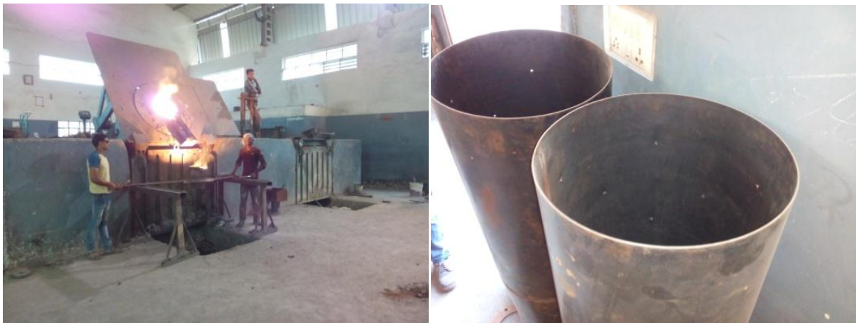
L-Melting furnace; R – existing former and optimally sized former
