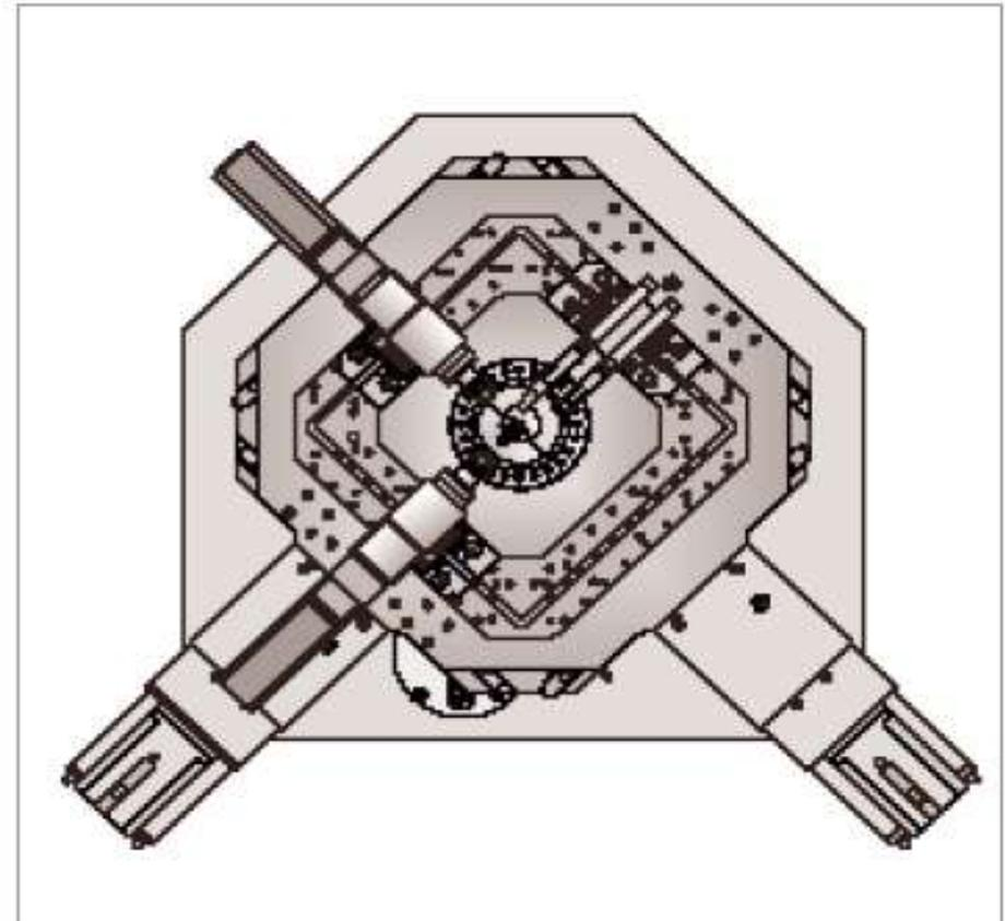
Basic machine with 6 CNC axes plus 1 rotary unit with switch mandrel
