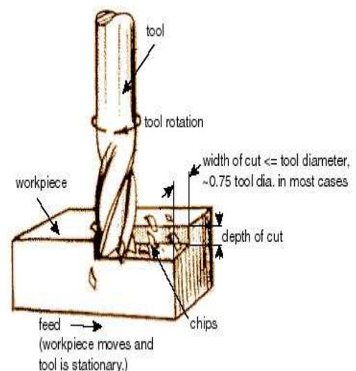
building, or company where machining is done is called a machine shop. Much of modern day machining is controlled by computers using computer numerical control (CNC) machining. Machining can be a business, a hobby, or both.
