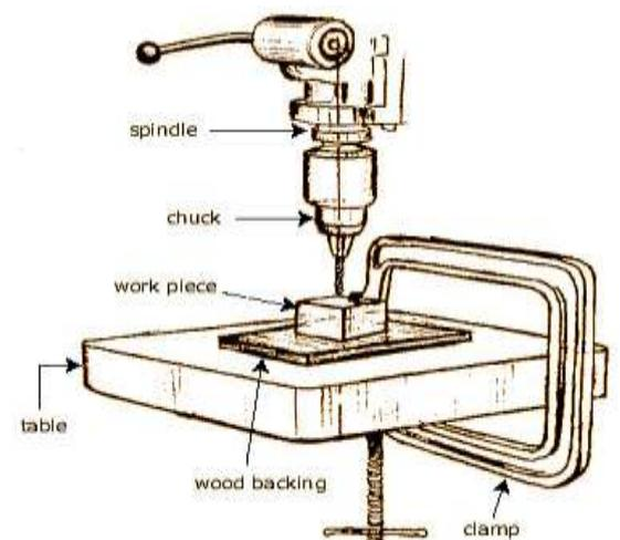
Drilled holes can be either through holes or blind holes. A through hole is made when a drill exits the opposite side of the work; in blind hole the drill does not exit the workpiece.
