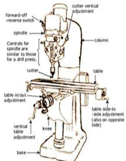
Milling is typically used to produce parts that are not axially symmetric and have many
