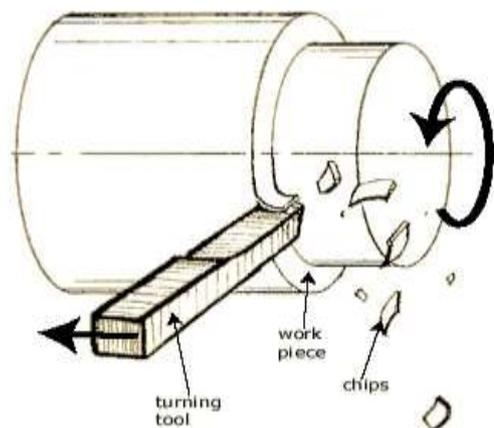
process to add or refine features on parts that were manufactured using a different process. Due to the high tolerances and surface finishes that turning can offer, it is ideal for adding precision rotational features to a part whose basic shape has already been formed.
