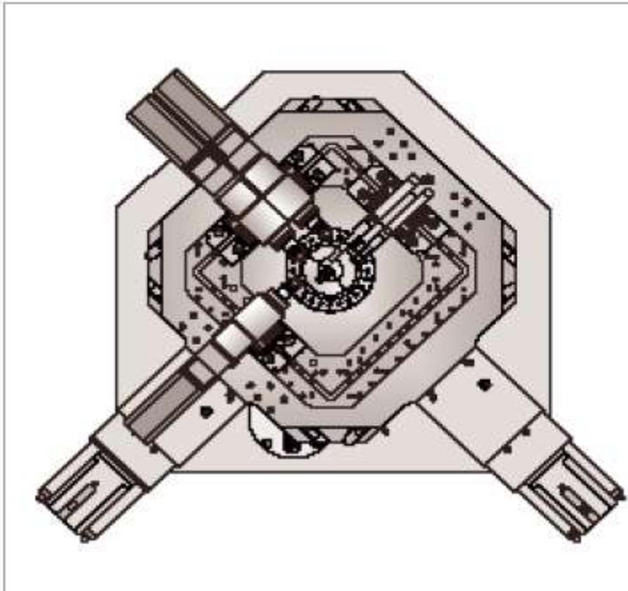
Basic machine with 6 CNC axes and 2 additional rotary units
