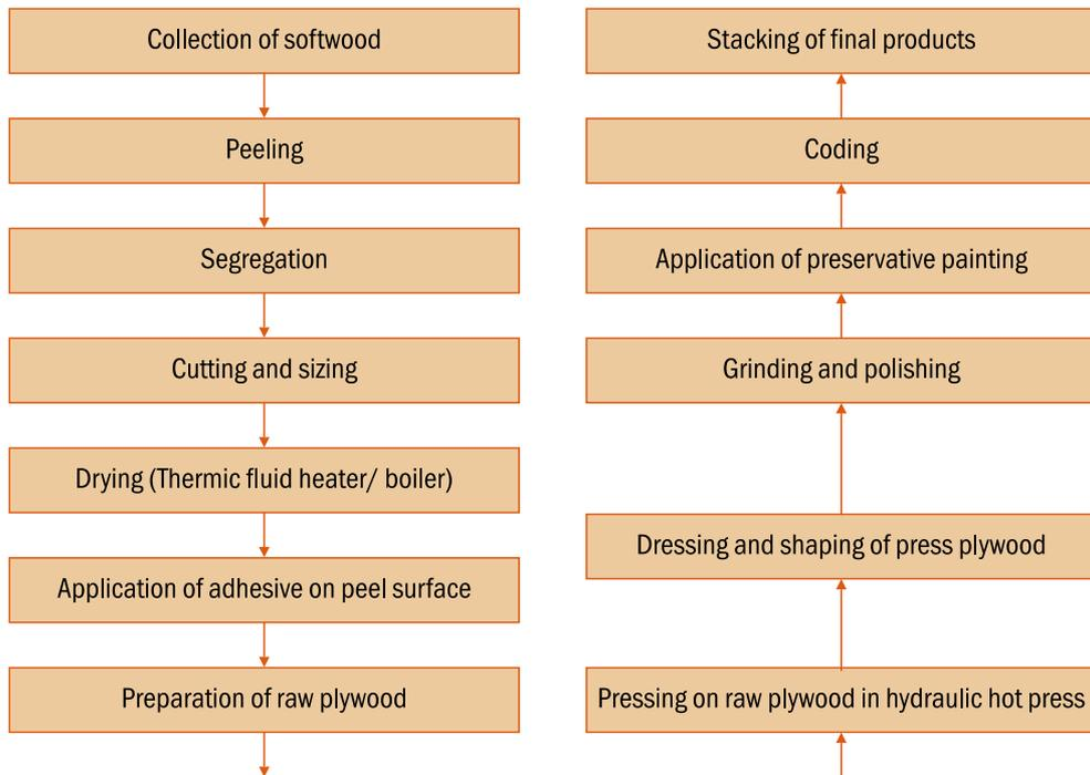
Process flow diagram of plywood manufacturing
