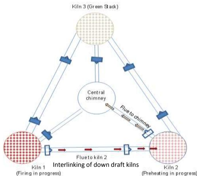
Figure: Schematic layout of integrated DD kilns with central chimney
