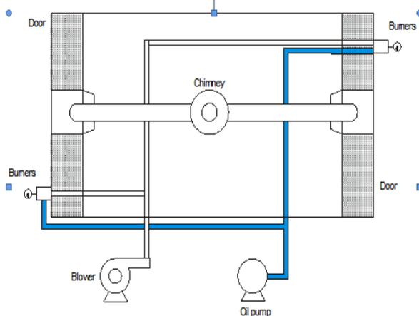
Schematic of tunnel kiln
