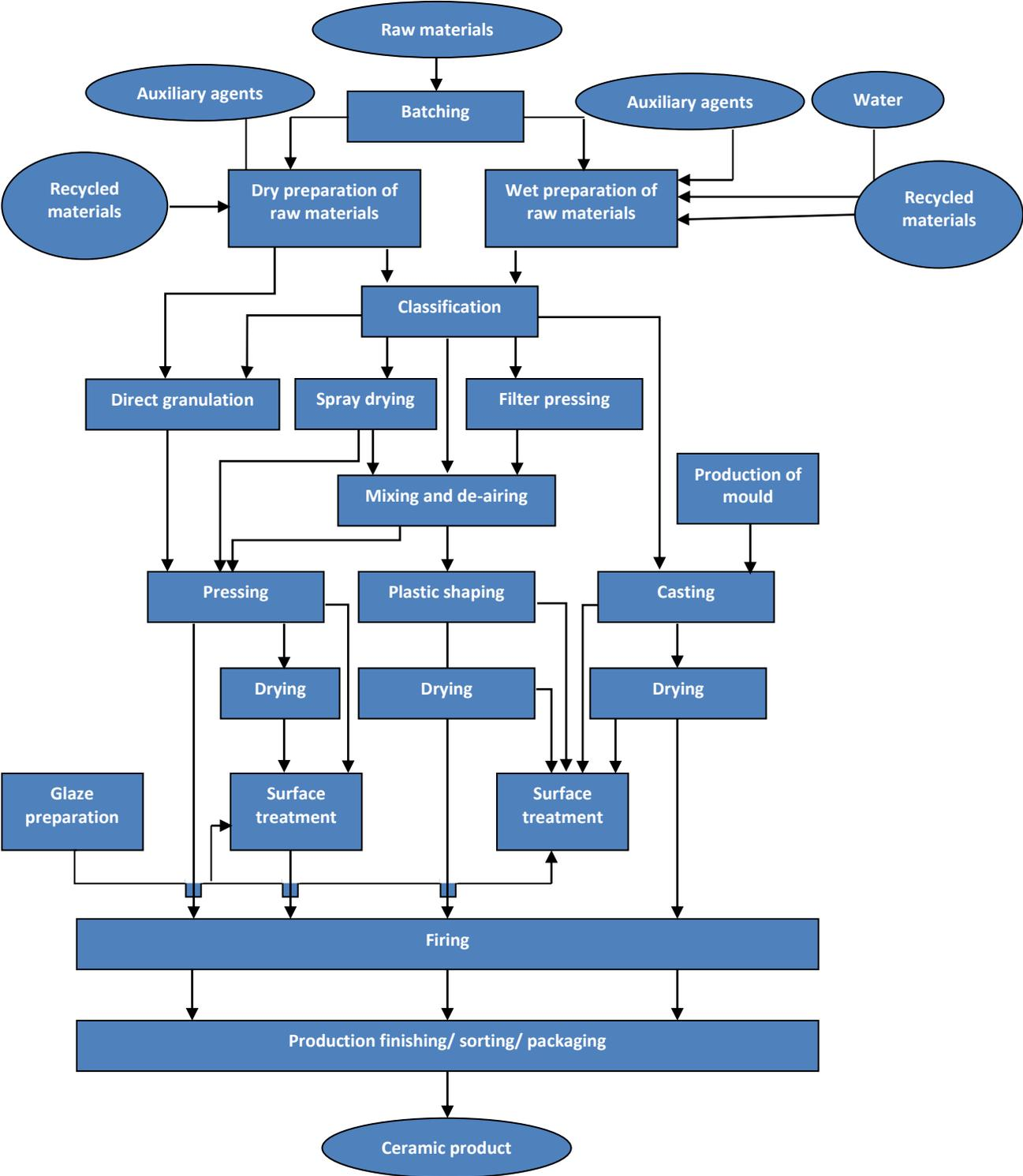
Typical process flow diagram of ceramic products
