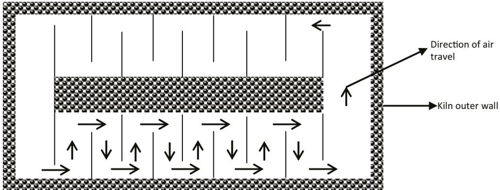
*Air flow in single zig-zag firing process*
