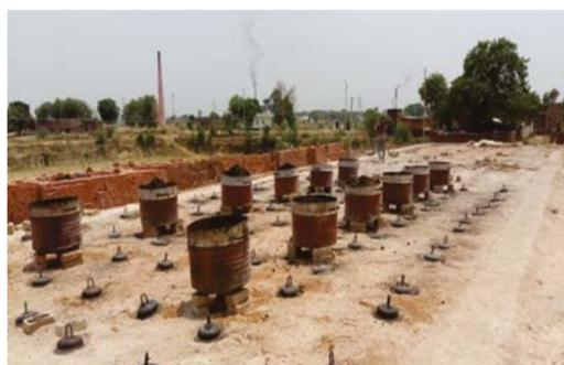
*Firing zone in zig-zag firing process*
