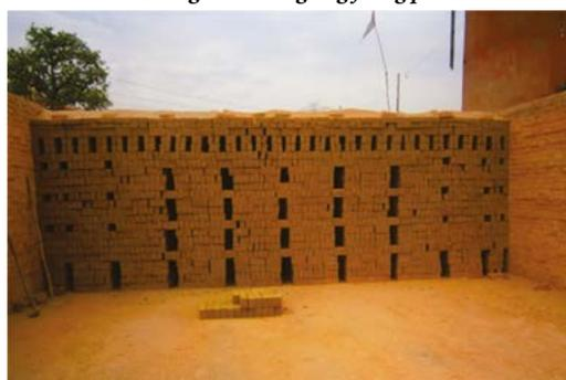
*Brick stacking in zig-zag firing process*
