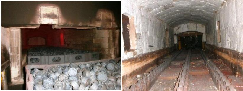
LPG-fired normalizing furnace: L- Before; R- After veneering
