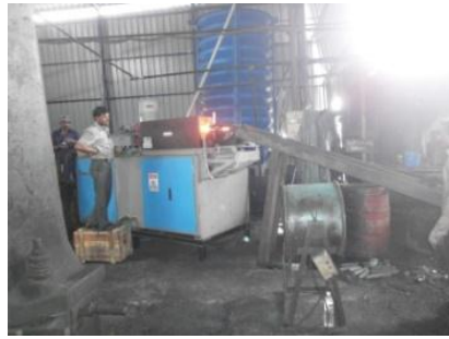
L- FO-fired furnace; R- Induction billet heater
