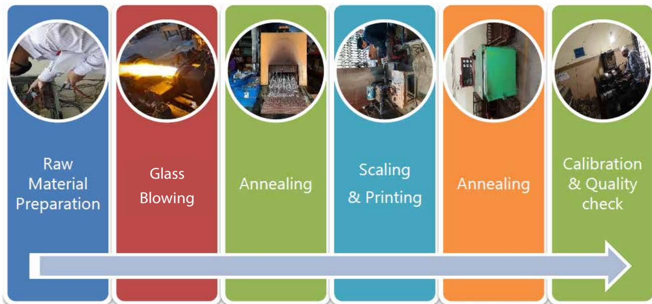
**Figure 1.** Basic stages in the lab glassware production process
