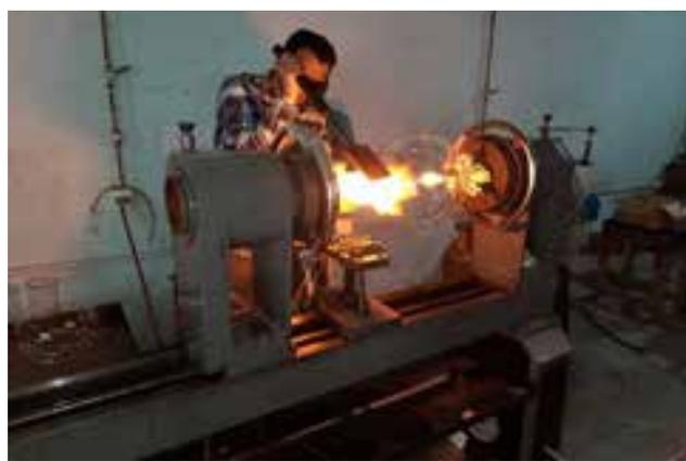
**Figure 2.** Glass blowing lathe
