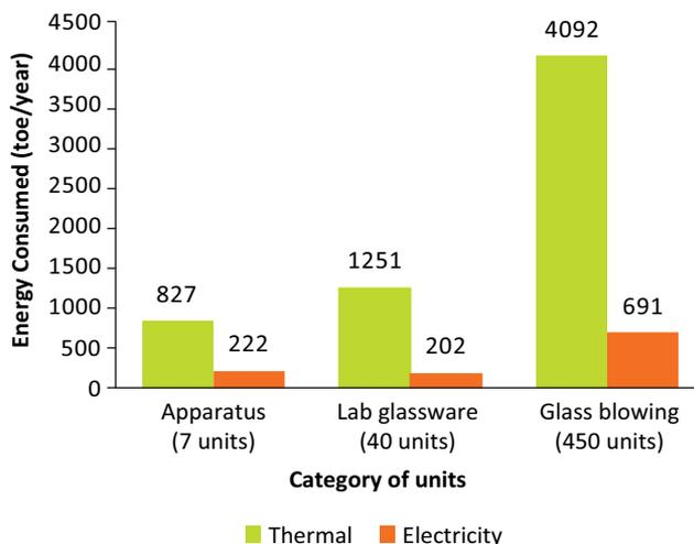
**Figure 4.** Energy consumption profile of Ambala laboratory glassware units
