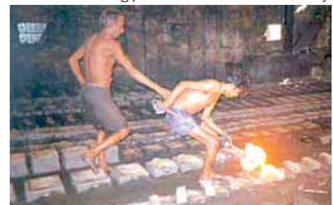
Molten metal being poured into moulds in a foundry
