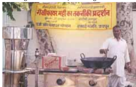
Biomass gasifier for food-processing unit
