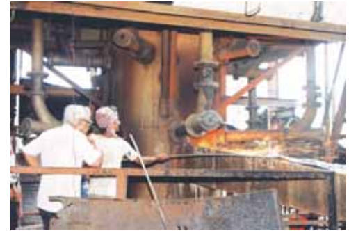
Divided blast cupola in a foundry
