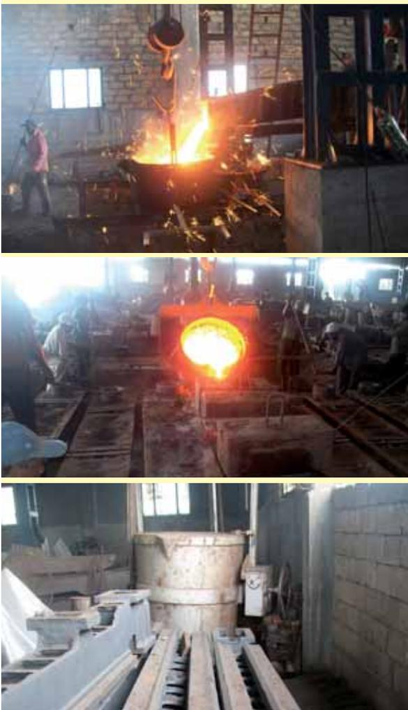
**Figure 10** 33-inch DBC commissioned at Carbo Tech: (a) Drawing molten metal from DBC; (b) Pouring metal into moulds; (c) Heavy lathe bed castings
