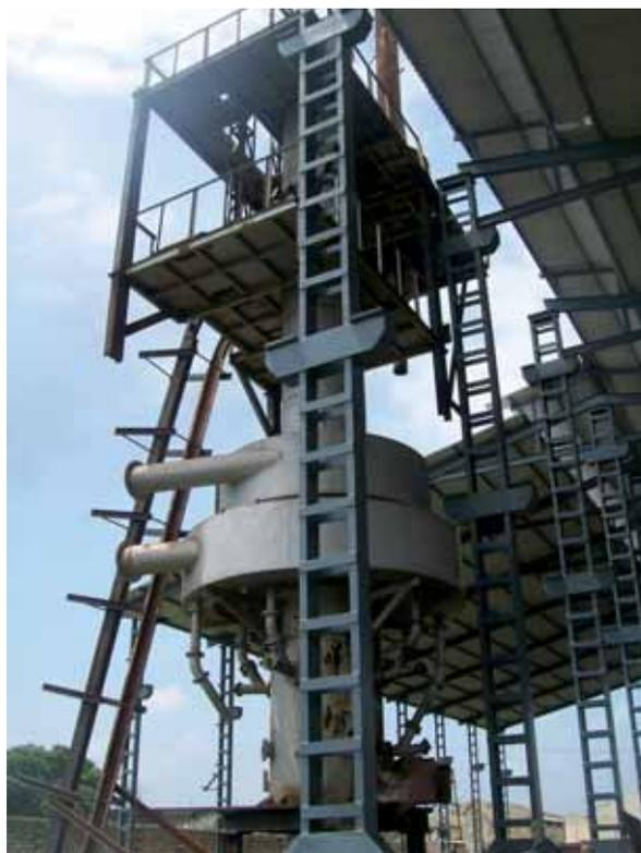
**Figure 8** New 21-inch DBC installed at Gautam Technocast
