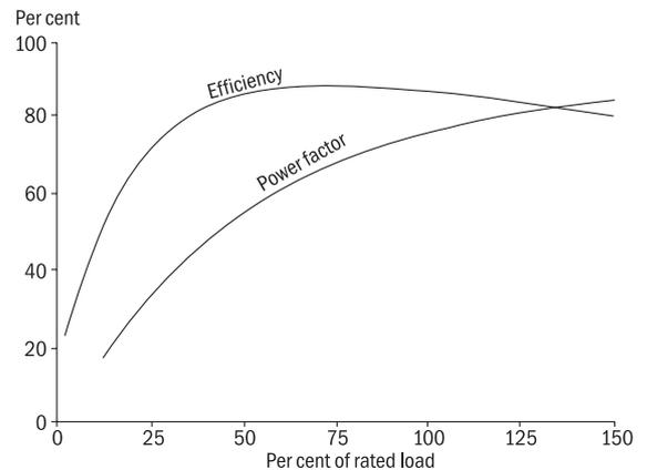
**Figure 3** Variation in efficiency and power factor with load on the motor
