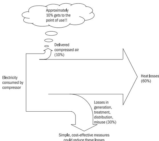
**Figure 3** Typical sankey diagram for a compressed air system
