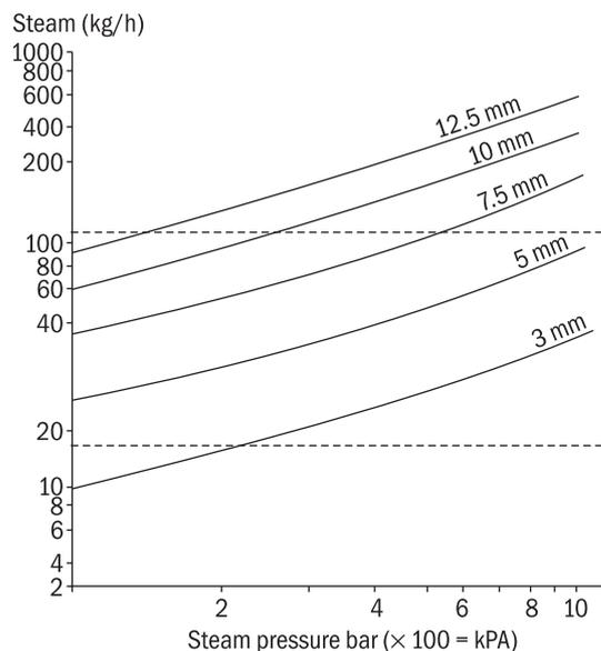
**Figure 2** Steam losses from various leakage sizes and pressure
